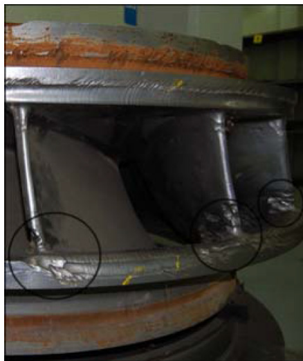
Erosion at runner outlet
